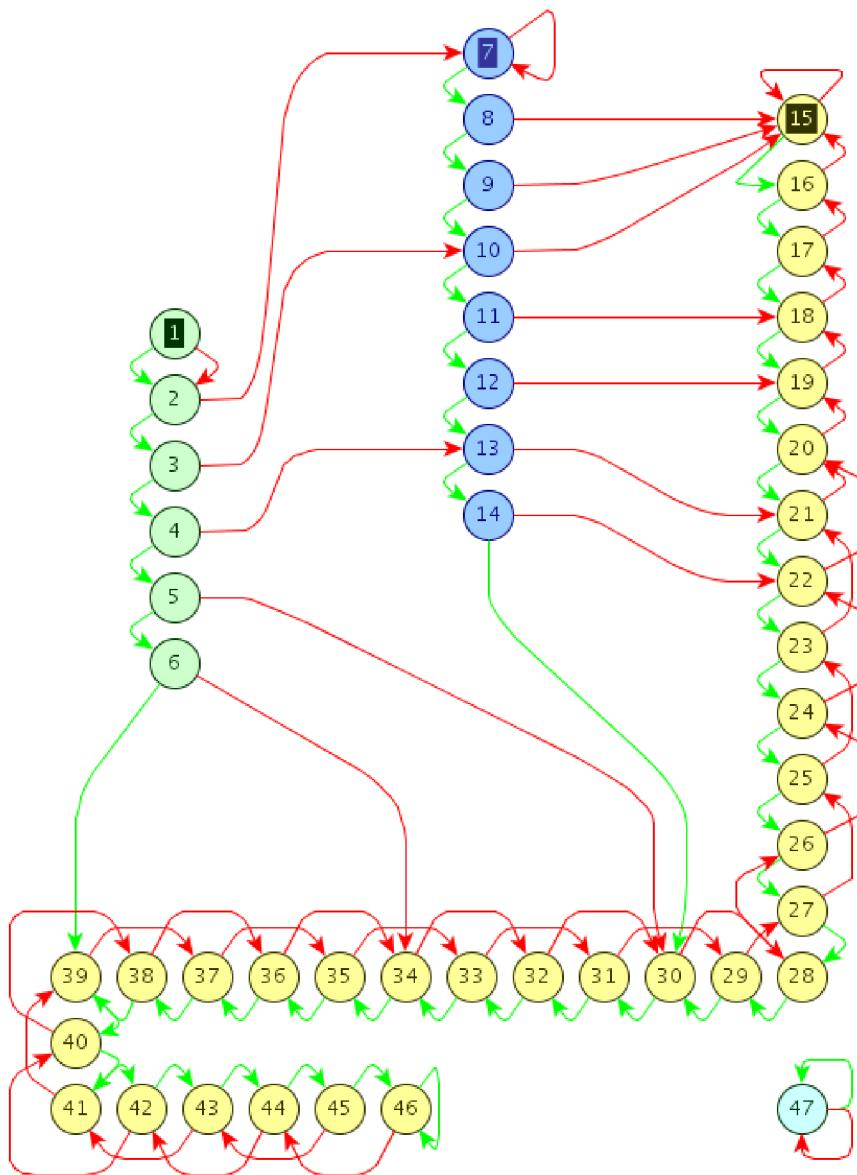
Figure 6.1: MQ coder state diagram.
