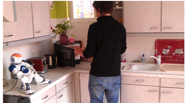
Fig. 1: This figure shows a robot companion, i.e., the humanoid robot NAO, listening to a person involved in an everyday kitchen activity. Using the continuous sound recognition method described in this paper, NAO is able to extract a discrete sequence of isolated sounds and to interpret them in terms of a pre-stored catalogue of auditory events (microwave alarm, open microwave door, close microwave door, toaster, etc.), all in the presence of background noise, competing sound sources, and reverberations. Remark how difficult would be to recognize this human activity using vision.
